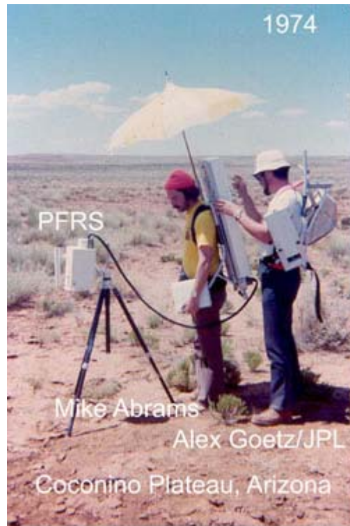
The whole PFRS unit of hardwired components, weighing about 40 lbs. Pictured here is ASD's co-founder Dr. Alex Goetz.
