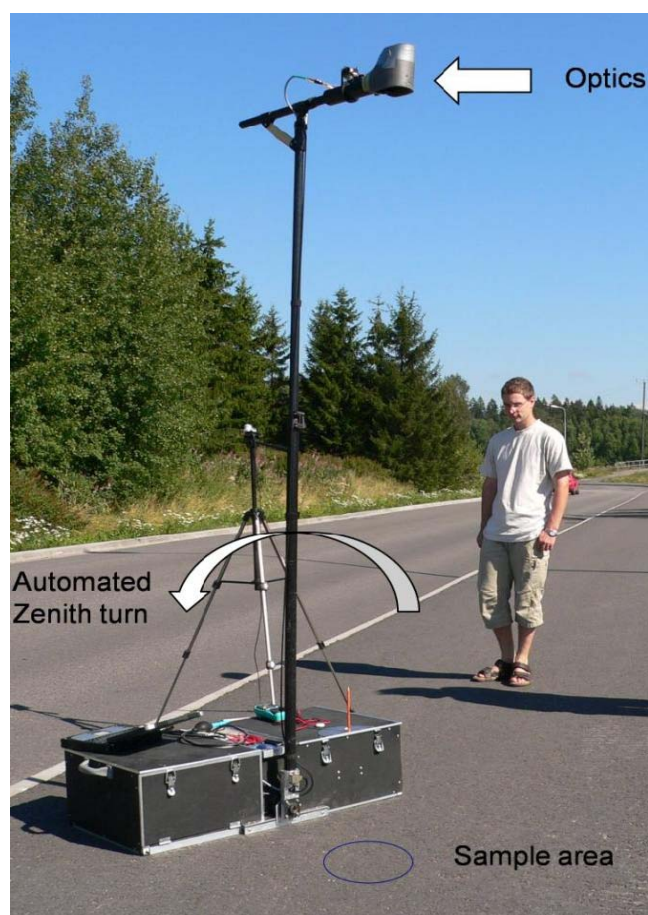
Figure 2. Finnish Geodetic Institute Field Goniospectrometer (FIGIFIGO) measuring asphalt reflectance. FIGIFIGO has automated zenith turn sequence, but it is manually rotated around the sample.
